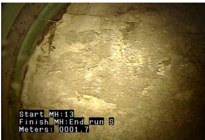
MSA - Survey Abandoned @ 1.7 m. Line plugged with concrete.
