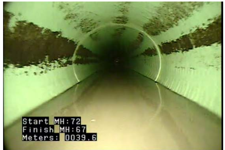
CL - Crack Longitudinal @ 39.6 m.
