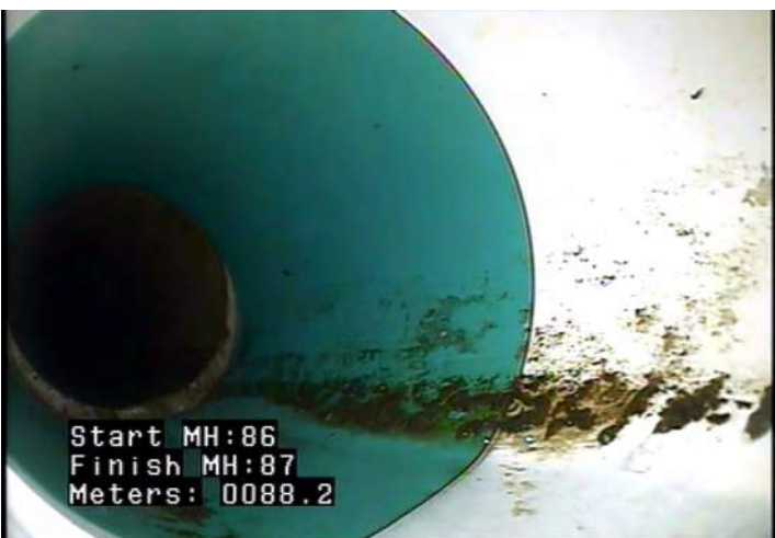
MSA - Survey Abandoned @ 88.2 m. Unable to pass bend
