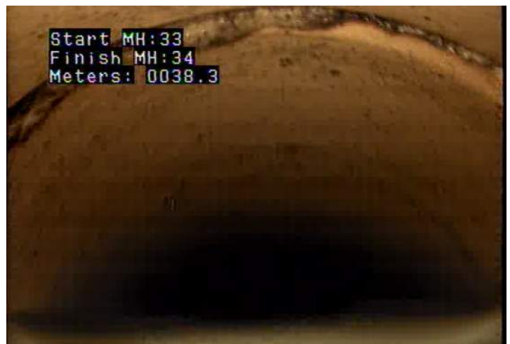
DAE - Deposits Attached: Encrustation @ 38.3 m.
