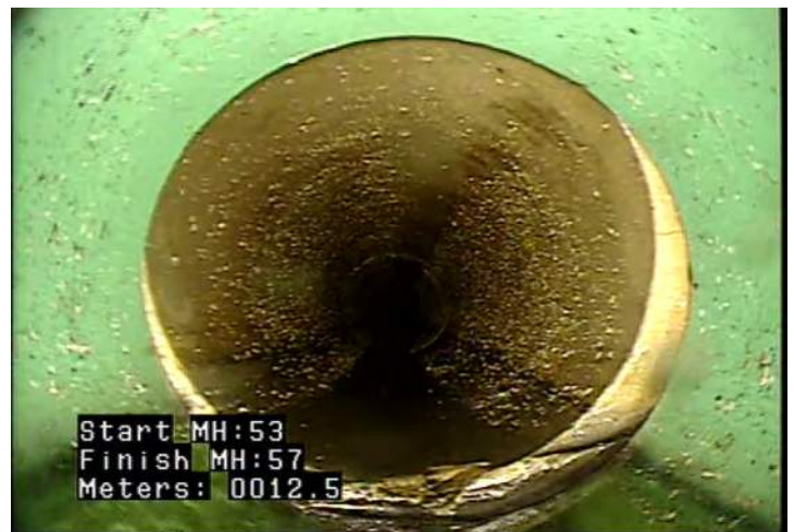
MMC - Material Change @ 12.5 m. PVC to Clay tile
