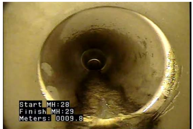
JOM - Joint Offset (displaced): Medium @ 9.8 m.
