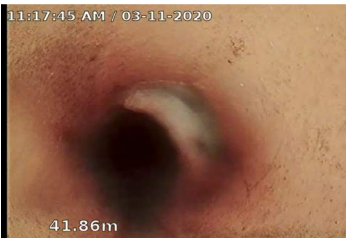
H - Hole in Pipe @ 41.9 m. Patched on outside
