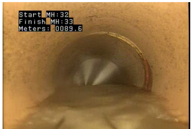
DAE - Deposits Attached: Encrustation @ 89.6 m.
