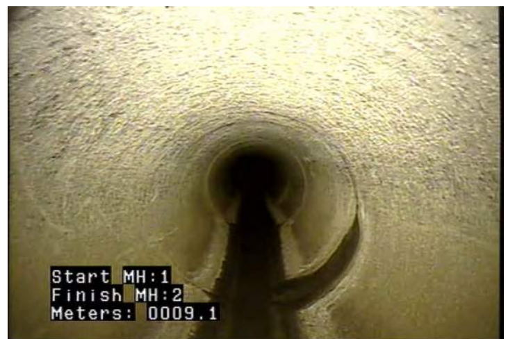
CC - Crack Circumferential @ 9.1 m.
