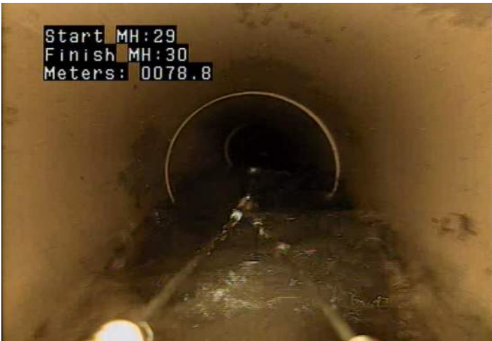
MWLS - Water Level: Sag @ 78.8 m.
