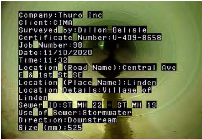
AMH - Access Point - Manhole @ 0.0 m. ST MH 22 - No access/Buried
