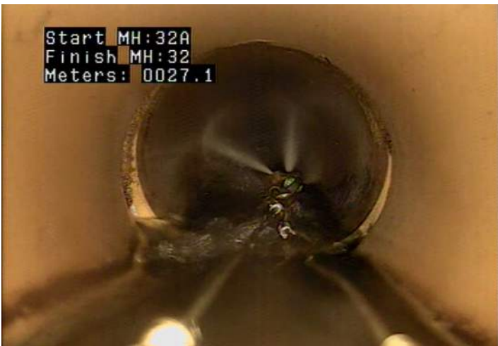
DAE - Deposits Attached: Encrustation @ 27.1 m.
