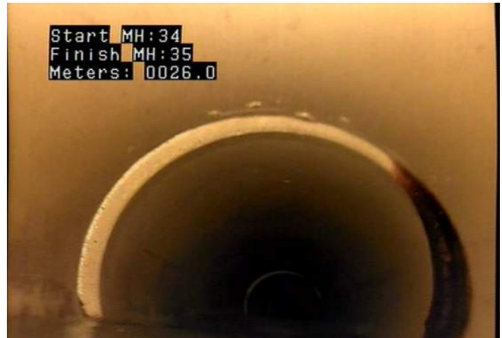
DAE - Deposits Attached: Encrustation @ 26.0 m.
