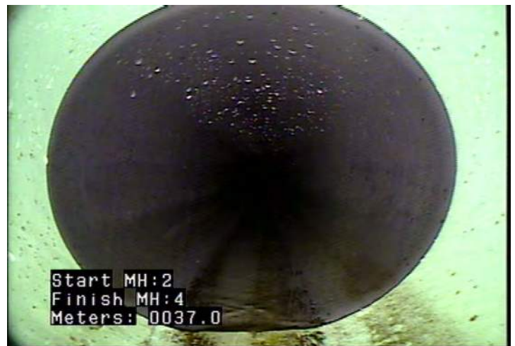
MMC - Material Change @ 37.0 m. Blue PVC to Grey PVC
