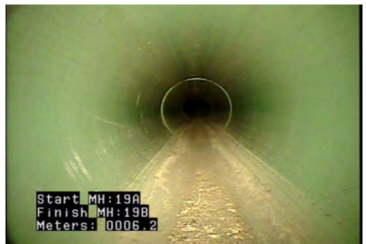
DSGV - Deposits Settled: Gravel @ 6.2 m.
