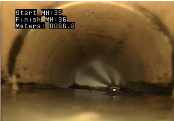
DAE - Deposits Attached: Encrustation @ 66.8 m.
