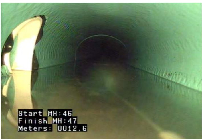
TSD - Tap, Saddle: Defective @ 12.6 m. Gasket intruding around service.
