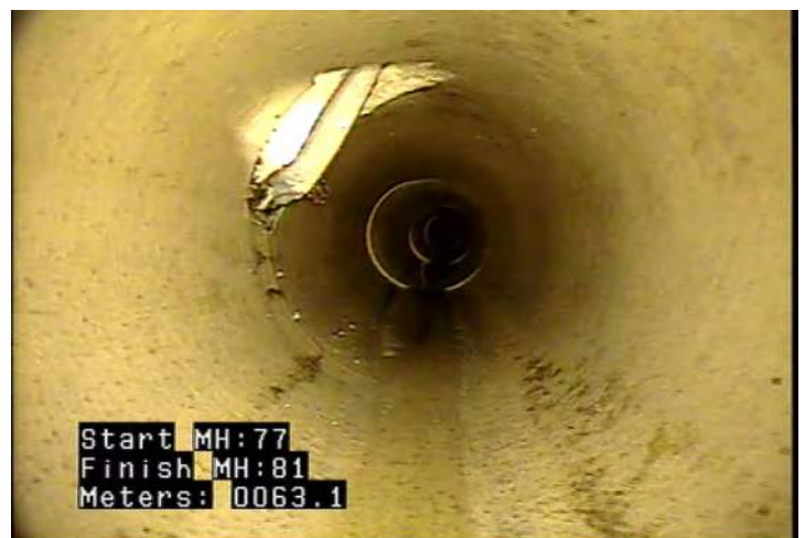
TBI - Tap, Break-in / Hammer: Intruding @ 63.1 m.
